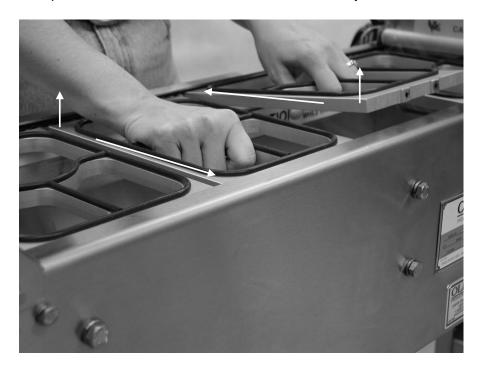
2.3. As the carriers are removed, the conveyor must be pulled forward to keep getting to the remaining carriers. To move the conveyor forward, grasp a tray carrier toward the infeed-end of the machine and pull the conveyor forward. This must be done with the conveyor disconnected from the drive (step 2.1).
