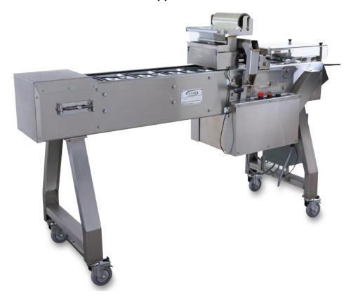
Remove the tie-downs that hold machine to the skid. Lift the machine off the skid in a safe manner. Remove tape and tie bands that were used to hold components for shipment.
