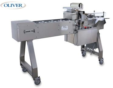
Weight:340 lb.Dimensions:width 78 x depth 23 x height 47 in.Maximum tray dimensions:8.6 x 6.5 x 3.25 in.Loading station:3 trays of 3 compartmentsNumber of tray carriers:14-20, depending on the tray modelElectricity:120 V AC, 6 A, 60 HzU.S. Patent Number:5,791,120
