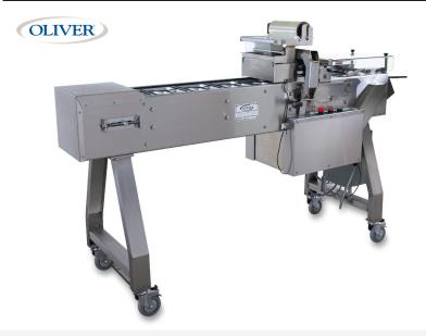
Weight: 340 lb. Dimensions: width 78 x depth 23 x height 47 in. Maximum tray dimensions: 8.6 x 6.5 x 3.25 in. Loading station: 3 trays of 3 compartments Number of tray carriers: 14-20, depending on the tray model Electricity: 120 V AC, 6 A, 60 Hz
